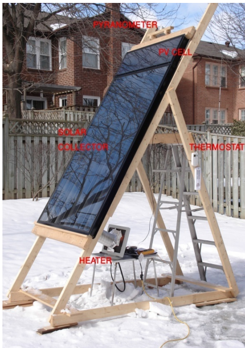
Figure 2.3: Test set up of the solar collector
